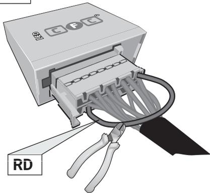
Pin 11 and Pin 2 disconnected
