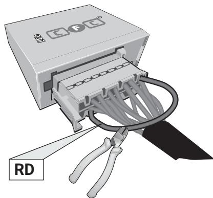
Pin 11 and Pin 2 disconnected
